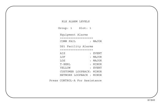
Figure 518-1. RLX Alarm Levels Screen (with Default Values)
